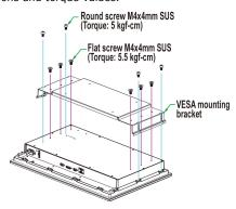
An additional four screws (not included in the kit) are required to mount the MPC-2000 series on a VESA rack. For this purpose, use M6 screws with a length between 10 and 12 mm.
