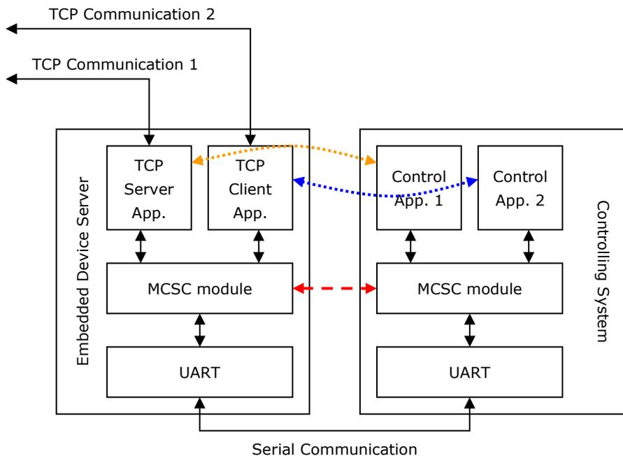
The MCSC module is built into the MiiNePort E1. To enable MCSC, you need to set your MiiNePort E1 serial port operation mode to MCSC mode and then set the channels' operation mode individually according to your application. In addition, you also need to implement the MCSC module in your device's primary system.
