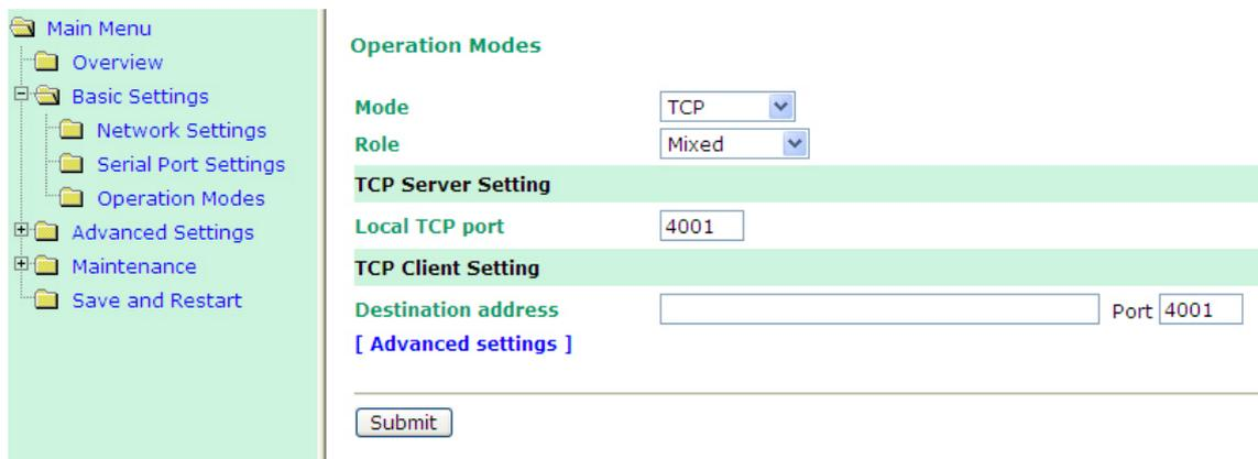
The screenshot shows the configuration interface for TCP Mixed Mode. On the left is a navigation menu with options: Main Menu, Overview, Basic Settings (expanded), Network Settings, Serial Port Settings, Operation Modes, Advanced Settings, Maintenance, and Save and Restart. The main content area is titled 'Operation Modes' and contains the following settings:
