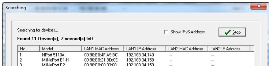
3. When the search is completed, all the located MiiNePort E1 modules will be displayed in the Device Search Utility window. Select the device you wish to access and press the **UnLock** button to input the password for the device. The default password is **moxa**.
