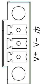
The UC-8100 has a 3-pin terminal block for a 12 to 24 VDC power input.
