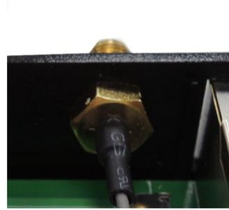
5. Install the connector; place the locking washer first, and then tighten the nut.
