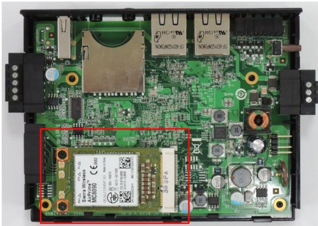
3. Next, you need to install the antenna cable. There are two antenna connectors on the cellular module. Connect the cable to either connector.
