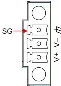
SG: The Shielded Ground (sometimes called Protected Ground) contact is the bottom contact of the 3-pin power terminal block connector when viewed from the angle shown here. Connect the SG wire to an appropriate grounded metal surface.
