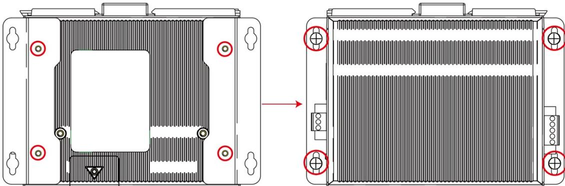
**NOTE** Before tightening the screws into the wall, make sure the screw head and shank size are suitable by inserting the screw into one of the keyhole-shaped apertures of the wall mounting plates.
