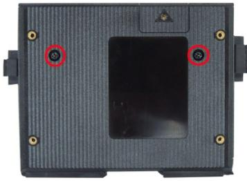
2. Find the location of the PCIe socket. Insert the cellular module into the socket, and then tighten the screws to fasten the socket.
