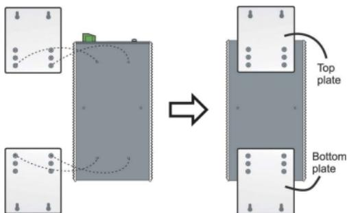
**STEP 2:** Mounting the EDS-510A on the wall requires 4 screws. Use the EDS-510A, with wall mount plates attached, as a guide to mark the correct locations of the 4 screws. The heads of the screws should be less than 6.0 mm in diameter, and the shafts should be less than 3.5 mm in diameter, as shown in the figure on at right.
