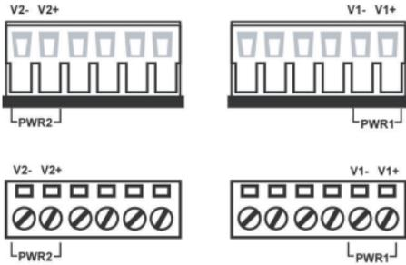
**STEP 1:** Insert the negative/positive DC wires into the V-/V+ terminals, respectively.
