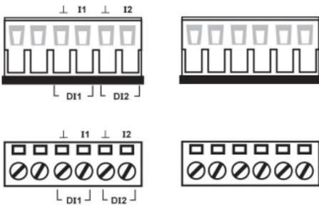
**STEP 1:** Insert the negative (ground)/positive DI wires into the  $\perp$ /I1 terminals, respectively.
