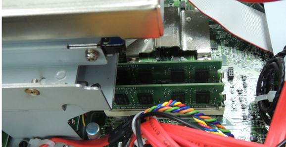
3. Simply push the two clutches on both sides of the memory module, and then remove the memory.
