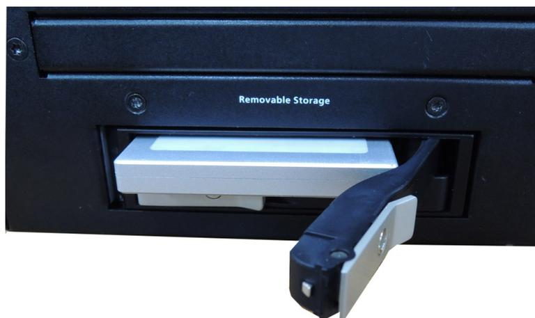
4. When finished, close the latch, and complete the installation by turning the key leftwards to lock the tray into place.
