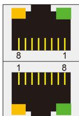
The LED indicators on the right-top (for the upper LAN connector) and right-bottom (for the lower LAN connector) corners glow a solid green color when the cable is properly connected to a 100 Mbps Ethernet network. The LED will flash on and off when Ethernet packets are being transmitted or received.
