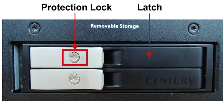
3. Pull out the protection lock and then directly insert the storage device, such as HDD or SSD, into the slot.
