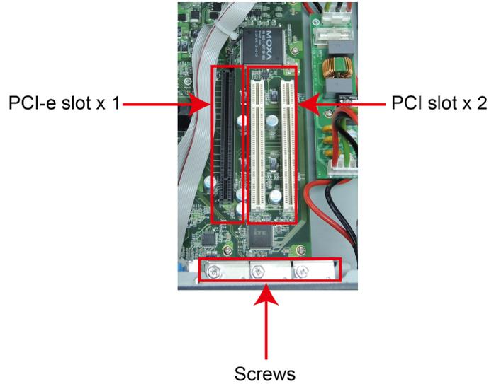
3. Remove the screws on the slot protection covers.
