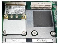
4. Attach the flat end of an antenna cable to the connector marked MAIN and insert the other end of the cable from the inside out into the antenna connector hole marked MAIN on the front panel of the computer using the antenna connector.
