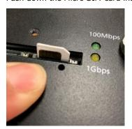
To remove the SIM card, push it down to release the card.
