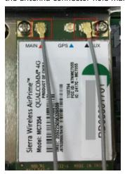
4. Use the black tape provided in the package to secure the antenna cables to the module. Attach tags (also provided in the package) to the cables as shown in the picture below to easily identify them.
