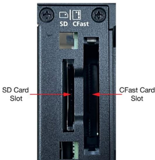
3. Insert the SD and CFast cards in the designated slots. Refer to the image printed beside the slots for the correct direction to insert the cards. When the cards are successfully inserted, you will hear a click.
