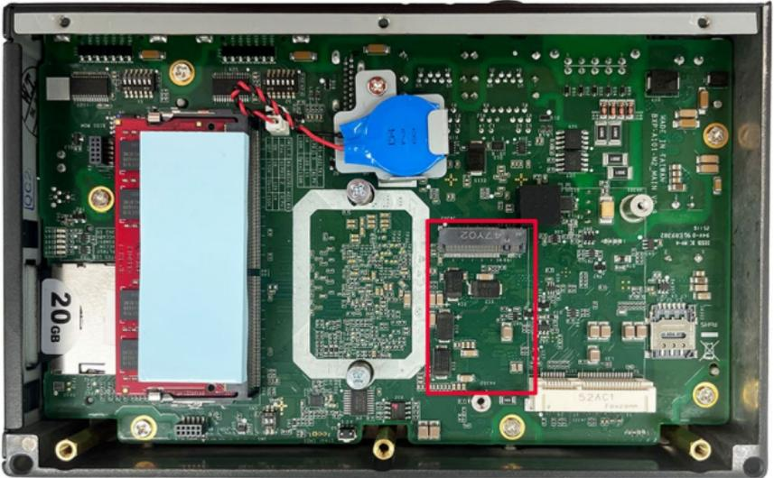
3. Install the M.2 module in the socket.
