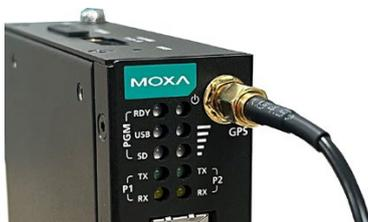
There are three antenna connectors on the front panel of the UC-2200A. W1 and W2 are for cellular modules. The GPS antenna connector is located on the top of the front panel. All three connectors are of SMA type.
