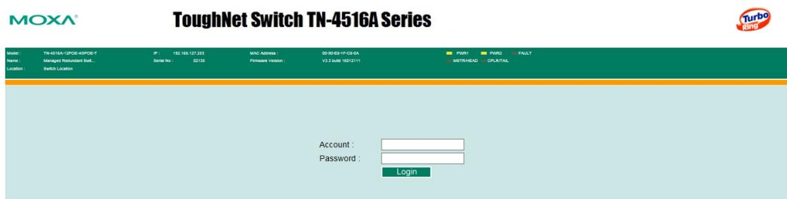
**NOTE** By default, the password assigned to the Moxa switch is moxa. Be sure to change the default password after you first log in to help keep your system secure.
