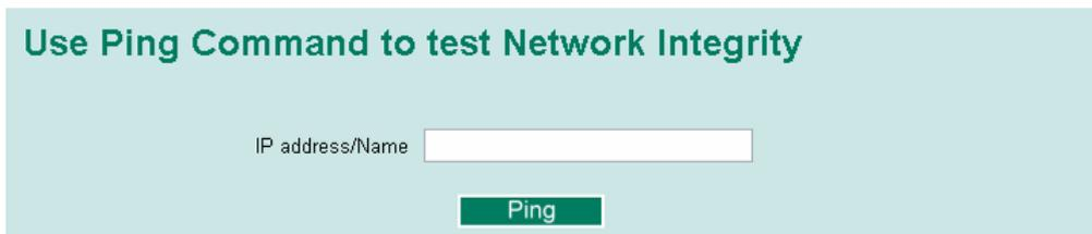
The **Ping** function uses the *ping* command to give users a simple but powerful tool for troubleshooting network problems. The function’s most unique feature is that even though the ping command is entered from the user’s PC keyboard, the actual ping command originates from the Moxa switch itself. In this way, the user can essentially sit on top of the Moxa switch and send ping commands out through its ports.
