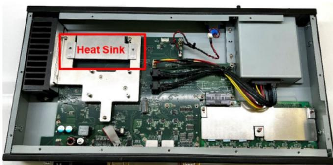
4. Remove the two M3x6 mm screws on the heat sink and remove the heat sink to reveal the memory slot.
