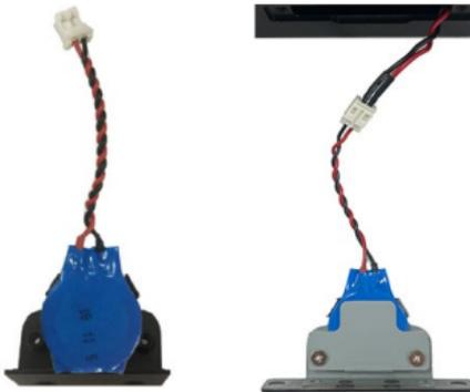
6. Plug in the connector of the battery-cover assembly to the internal wire of the slot.
