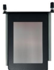
4. Reverse the storage tray and fasten four screws to secure the storage drive to the tray.
