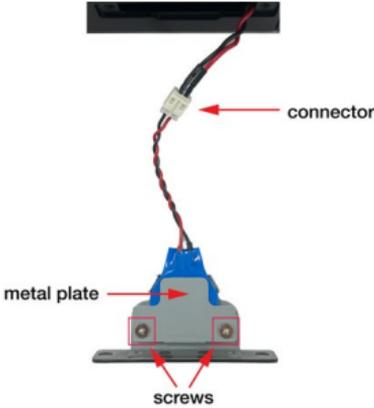
3. Unplug the connector of the battery-cover assembly from the internal wire of the slot.
