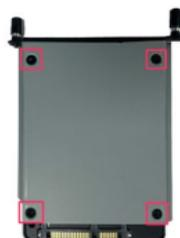
5. Insert the storage tray into the slot and fasten secure the tray in place with two screws.
