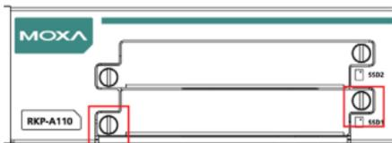
2. Pull out the storage tray and layout four screws from the pouch included in the product package.
