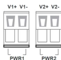
**STEP 1:** Insert the negative/positive DC wires into the V-/V+ terminals, respectively.
