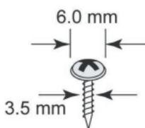
**NOTE** Before tightening the screws into the wall, make sure the screw head and shank size are suitable by inserting the screw through one of the keyhole-shaped apertures of the Wall Mounting Plates.
