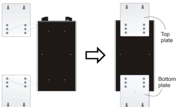
**STEP 2**—Mounting the EDS-P510A-8PoE on the wall requires 4 screws. Use the EDS-P510A-8PoE, with wall mount plates attached, as a guide to mark the correct locations of the 4 screws. The heads of the screws should be less than 6.0 mm in diameter, and the shafts should be less than 3.5 mm in diameter, as shown in the figure on at right.
