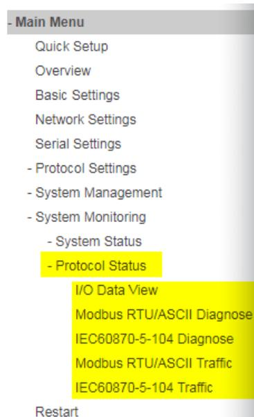
In the “**IEC 60870-5-104 Diagnose**” web page, we can monitor IEC 60870-5-104 Server connection status and the Object Points status.
