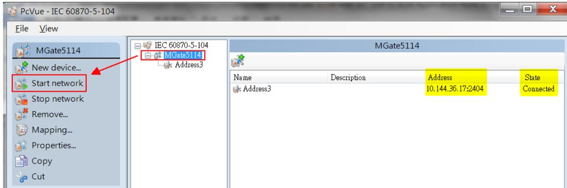
Click **Mapping** and an IEC 60870-5-104 object window will pop up. You can see several object points that are detected by the PcVue after making a connection according to the IEC 60870-5-104 communication characteristics. The objects include single-point information, double-point information, etc. They should be the same IEC 60870-5-104 server objects (MGate 5114).
