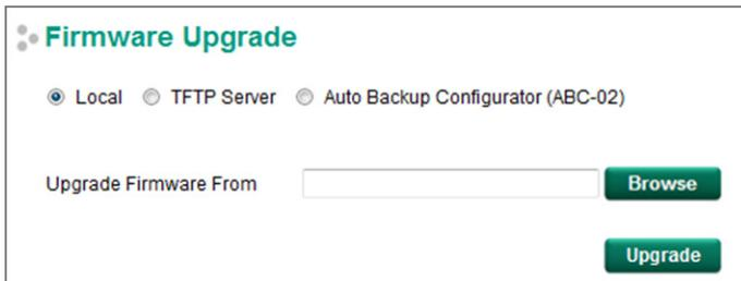
The screenshot shows the 'Firmware Upgrade' section of a web interface. At the top, there are three radio buttons: 'Local' (selected), 'TFTP Server', and 'Auto Backup Configurator (ABC-02)'. Below the radio buttons, there is a text input field labeled 'Upgrade Firmware From' and a green 'Browse' button to its right. Below the input field, there is a green 'Upgrade' button.
