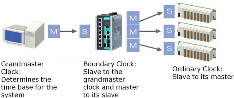
1. The **Boundary Clock and Transparent Clock** functionalities defined by IEEE 1588 must be implemented in the switch.
