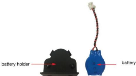
5. Place a new battery in the battery holder, replace the metal plate, and fasten the two screws on to the frame to secure the battery.
