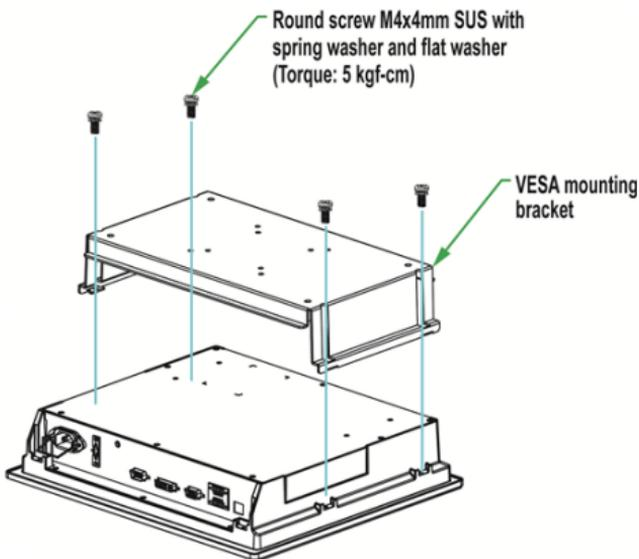
An additional four screws (not included in the kit) are required to mount the display on a VESA rack. Use M6 screws with a length between 10 and 12 mm for this purpose.
