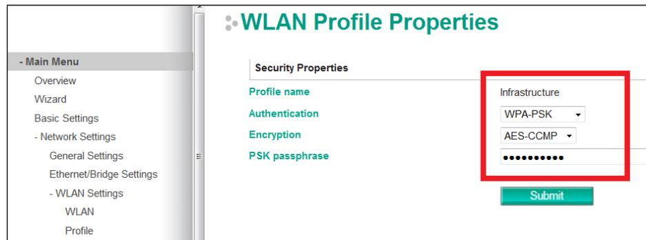
7.3.3. Save all the settings and restart the NPort W2x50A. Disconnect the Ethernet cable before booting up to enable the wireless connection. From the Cisco controller, check that the NPort W2x50A has successfully established a connection with the Cisco AP.
