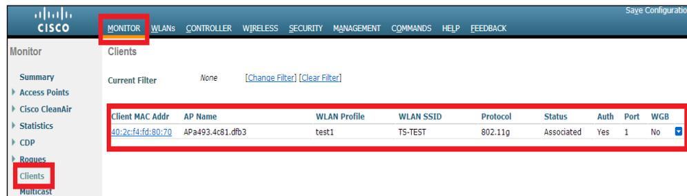
The screenshot shows the Cisco WLC Monitor page. The 'MONITOR' tab is selected. The 'Clients' section is active, showing a table of connected clients. The table has columns for Client MAC Addr, AP Name, WLAN Profile, WLAN SSID, Protocol, Status, Auth, Port, and WGB. A red box highlights the first row of data.
