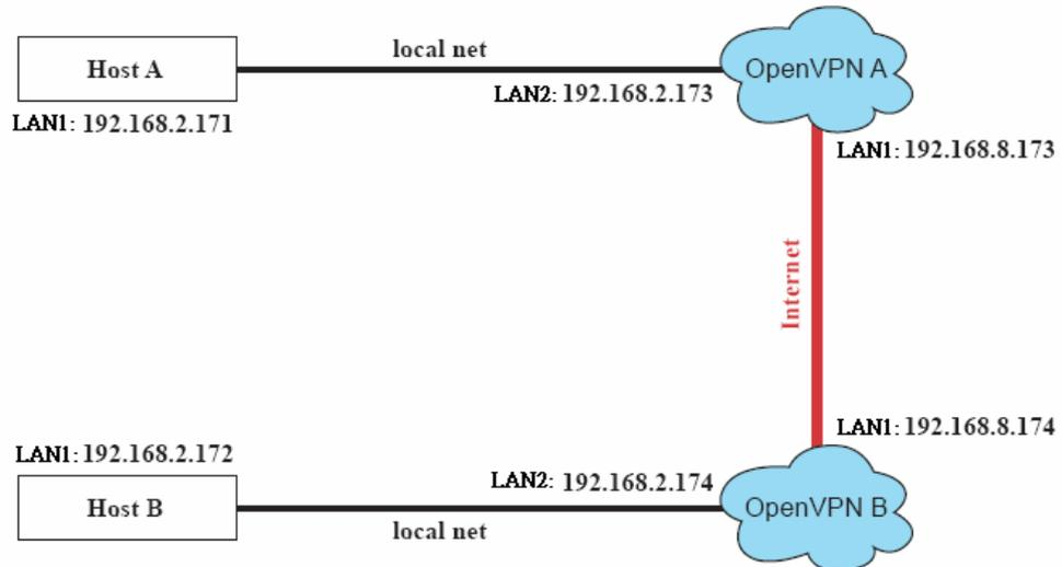
2. The configuration procedure is almost the same as for the previous example. The only difference is that you will need to comment out the parameter **up** in **/etc/openvpn/tap0-br.conf** of OpenVPN A and **/etc/openvpn/tap0-br.conf** of OpenVPN B.
