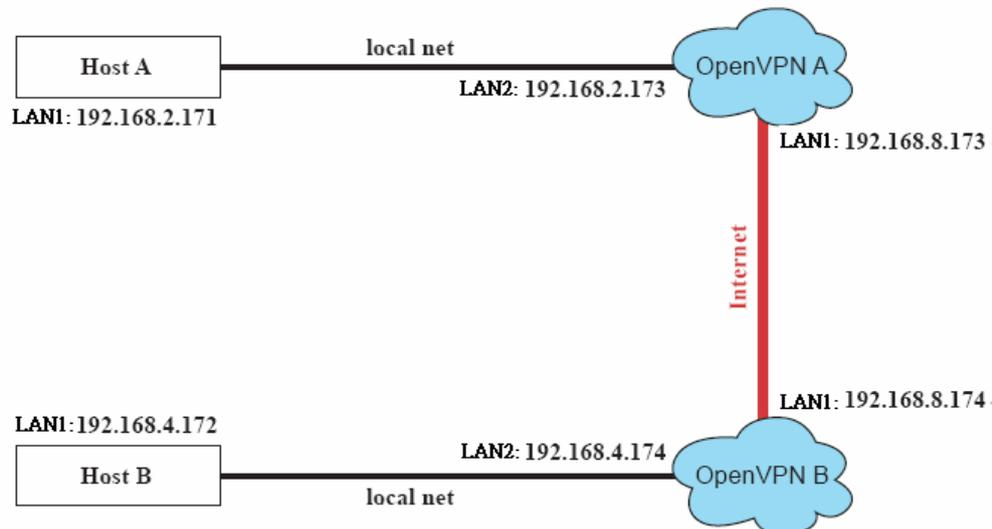
2. On machine OpenVPN A, modify the remote address in configuration file `/etc/openvpn/tun.conf`.
