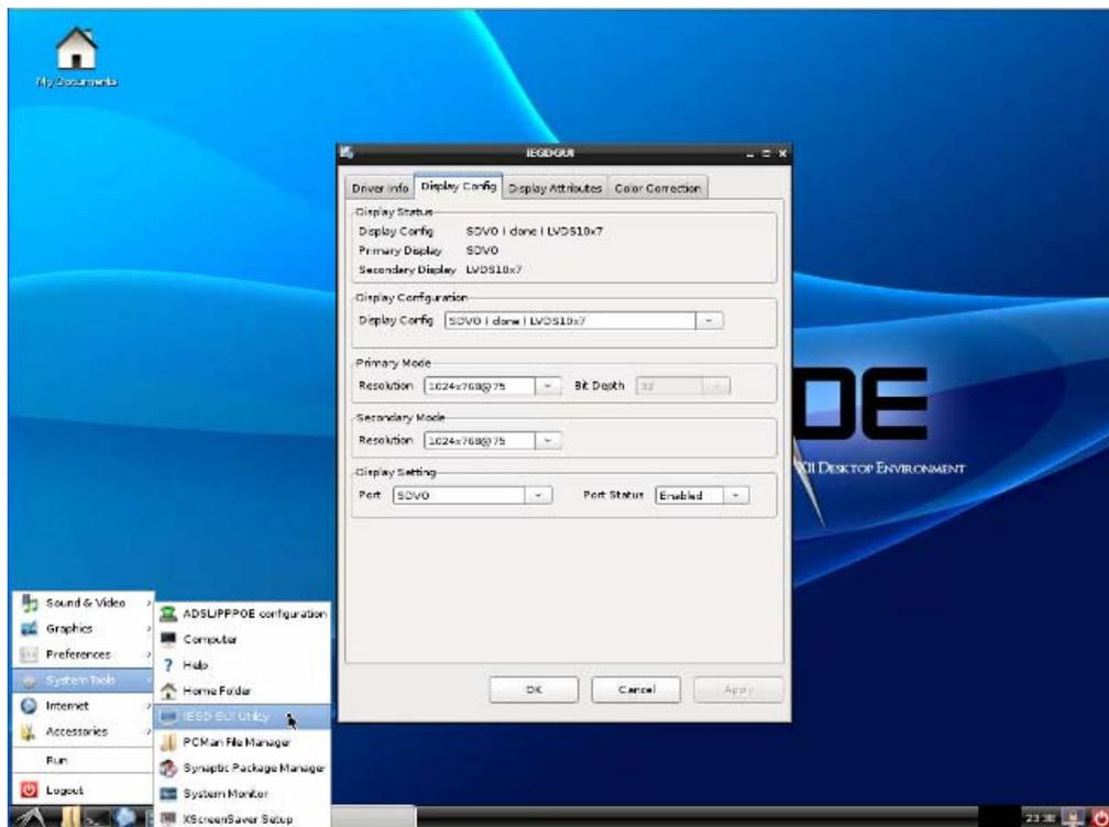
The V2101 IEGD driver supports three display configuration modes: **SDVO (single)**, **LVDS (single)**, **SDVO(clone)LVDS**. You may choose the display interface in this step. Note that the default setting is SDVO (clone)LVDS. In this mode, the setting of LVDS output will follow the SDVO mode.
