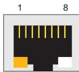
The bottom left corner LED indicator maintains a solid orange color when the cable is properly connected to a 10 Mbps Ethernet network. The LED will flash on and off when Ethernet packets are being transmitted or received.
