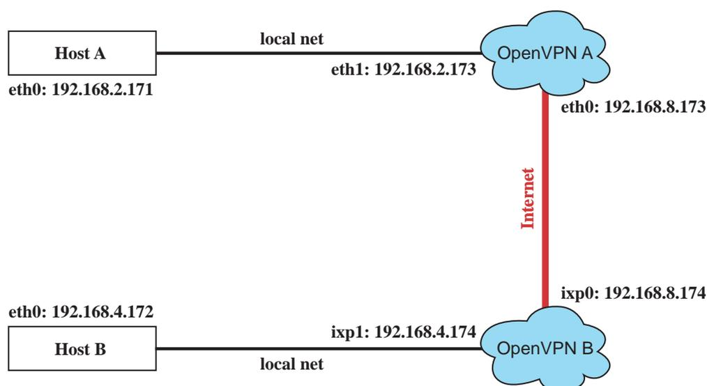
Host A (B) represents one of the machines that belongs to OpenVPN A (B). The two remote subnets are configured for a different range of IP addresses. When this setup is moved to a public network, the external interfaces of the OpenVPN machines should be configured for static IPs, or connect to another device (such as a firewall or DSL box) first.
